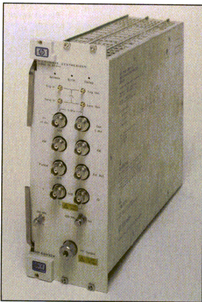
1. The E6432A VXI microwave frequency synthesizer covers a range of 10 MHz to 20 GHz with 1-Hz resolution and an assortment of modulation formats.
